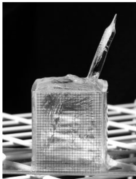
Fig. 2. Ice spike grown using distilled water in a Lexan container. A millimeter-scale grid is affixed to the front surface of the container.
