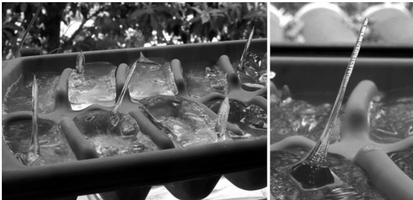
Fig. 1. A number of ice spikes grown in an ordinary plastic ice-cube tray using distilled water. Note the spikes grow at many different positions and angles and to various heights up to \approx 50 mm.
